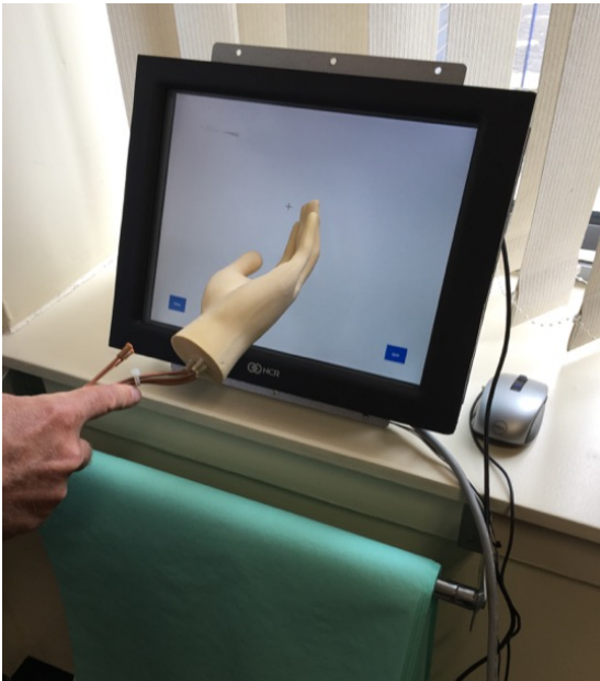
Figure 1: Prosthesis being held with simulated skin contact
