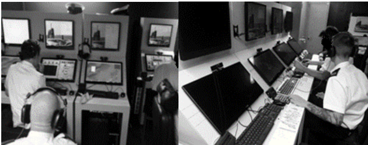
Figure 1: The ComTET submarine control room simulator, with sound room on the left hand side and picture room on the right
