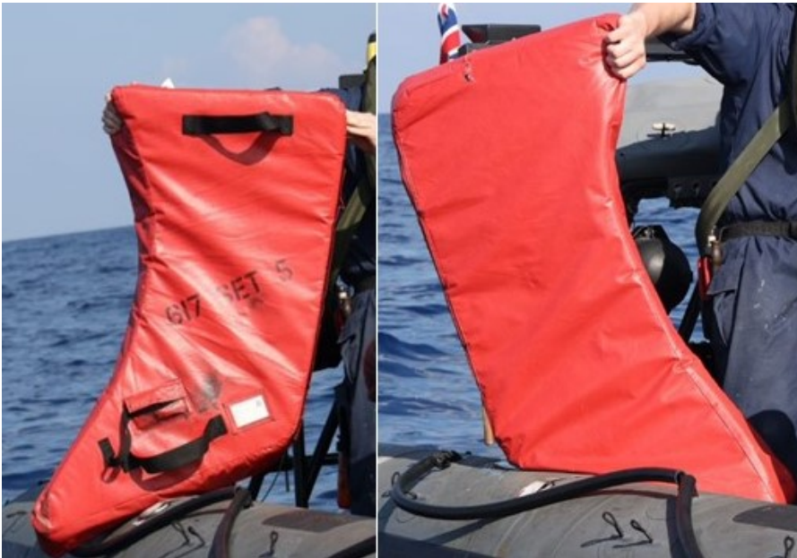
Figure 3: Left intake blank recovered from the sea.
