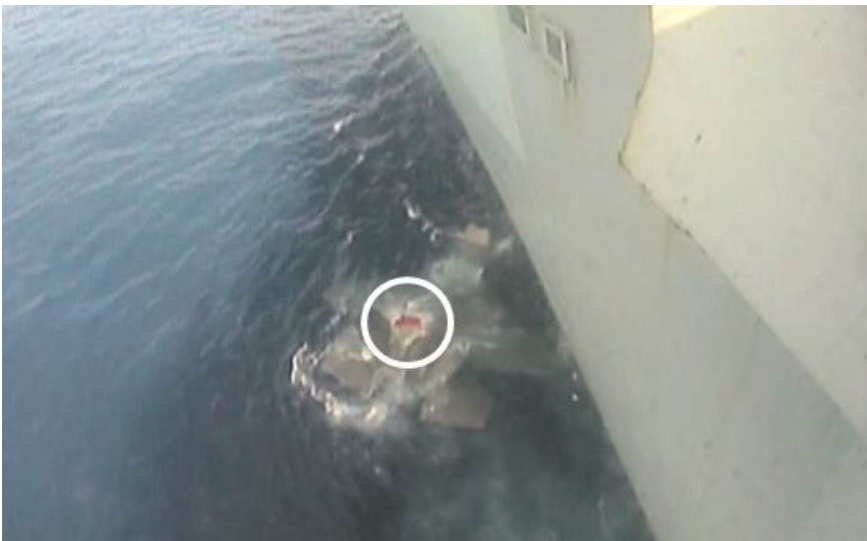
Figure 2: Left Intake blank floating out of the BK18's Auxiliary Inlet.
