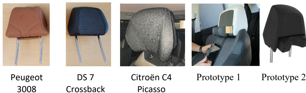
Figure 1: Headrests of the Peugeot 3008, Citroën C4 Picasso, DS7 Crossback and two newly developed prototypes
