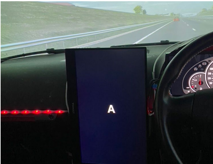
Figure 3: Interior of car showing forced distraction task and red lead vehicle visible on road ahead
