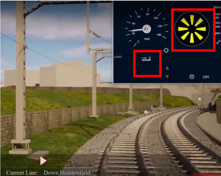
Figure 2: DMI ETCS transition announcement indicator and AWS task conflict
