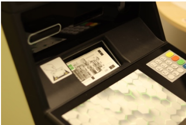
Figure 7: Cash inserted incorrectly (long edge first)
