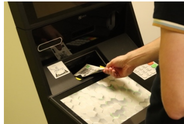
Figure 8: Cash inserted incorrectly (short edge first)
