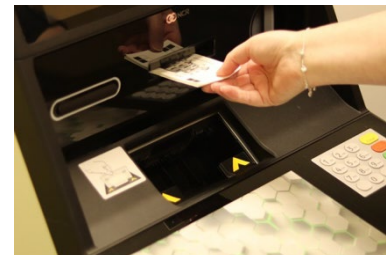
Figure 9: Cash inserted into wrong fascia location
