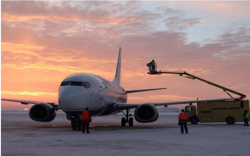
Figure 1 – Aircraft De-icing Procedure
