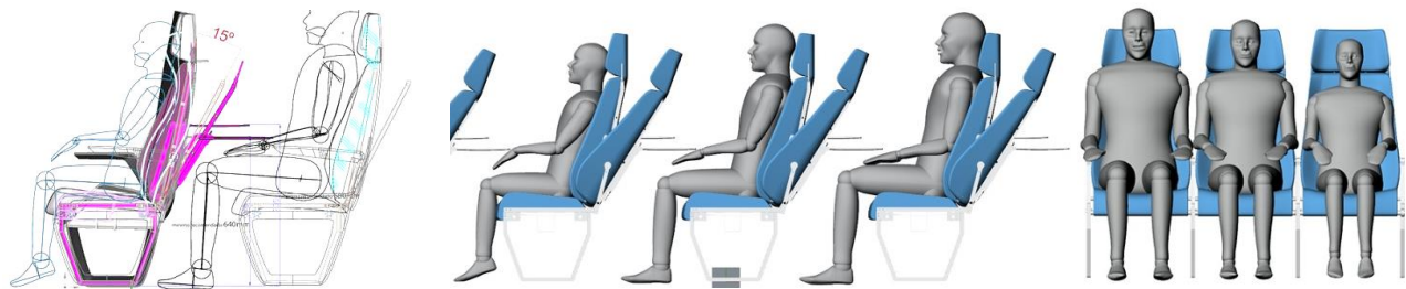
Figure 2: Virtual model ergonomic verification with seat structure 15°
