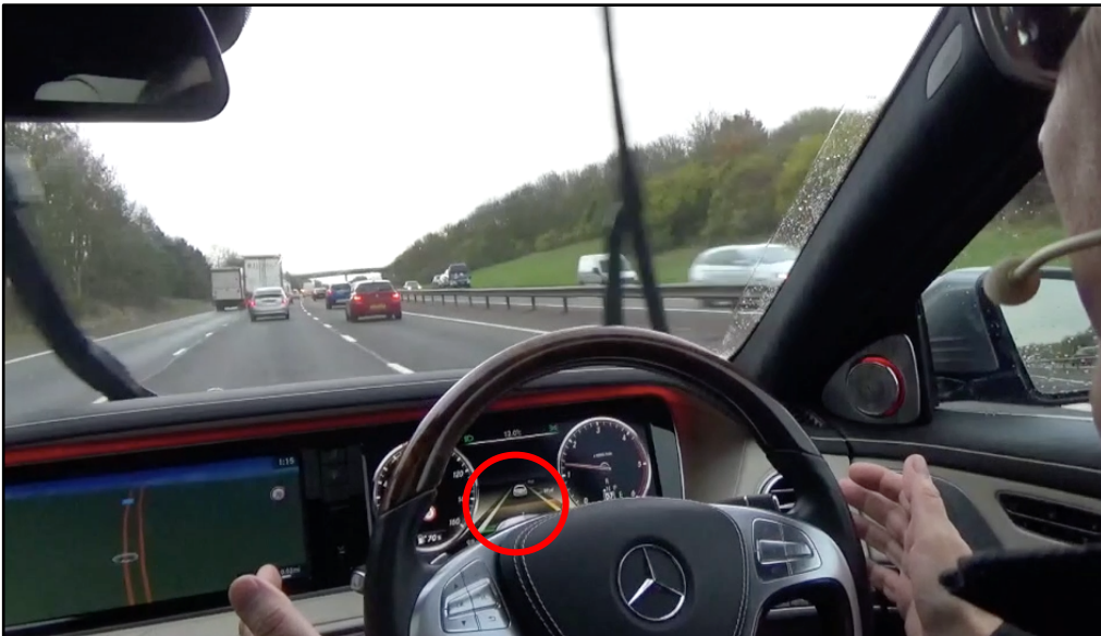
Figure 2: Showing Distronic Plus is correctly representing the outside world but is yet to reduce the headway (see within red circle) as it had increased after the red car in front had moved to the right hand lane.
