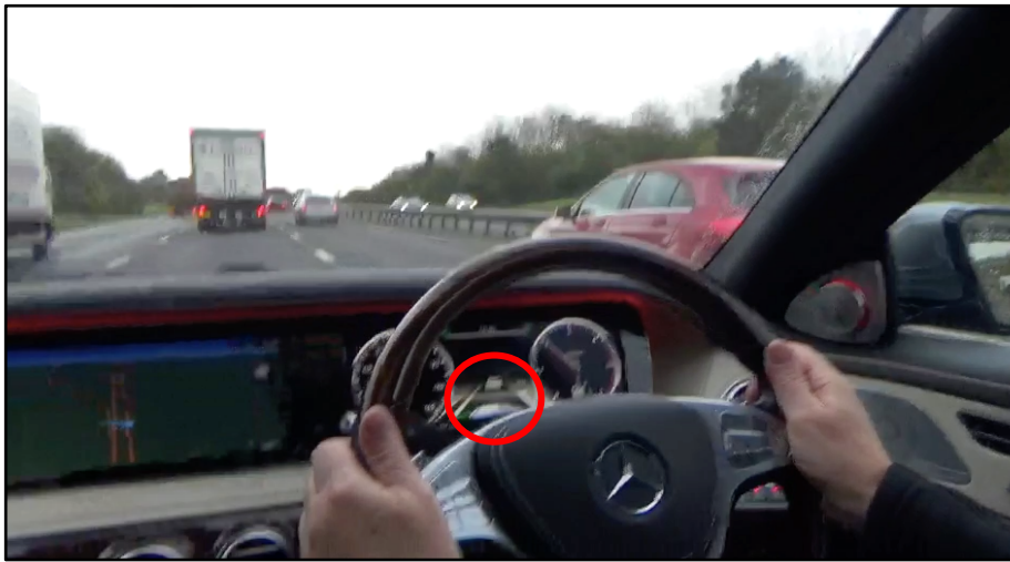
Figure 3: Showing the instant of manual braking when the driver lost confidence in the operation of the DISTRONIC PLUS. Within the red circle it can be seen that the Lorry has been sensed and the headway has not been breached, indicating correct functioning.
